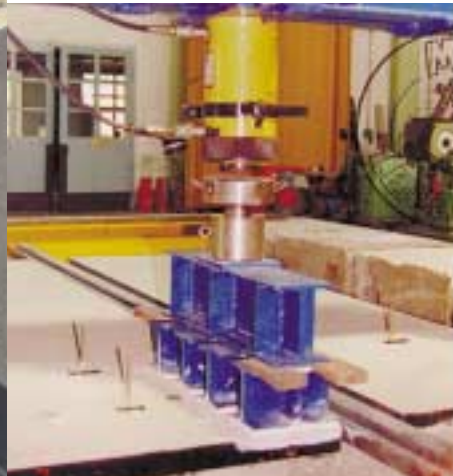
MfPA Leipzig, lab testing of slabs
